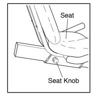
the console when you pedal. To adjust the seat, first turn the seat knob counterclockwise two or three turns to loosen it (if the seat knob is not loosened enough, the seat knob may scratch the frame). Next, pull the seat knob, slide the seat to the desired position, and release the seat knob. **Make sure to move the seat back and forth slightly until it locks in position.**Then, turn the seat knob clockwise to tighten it.
